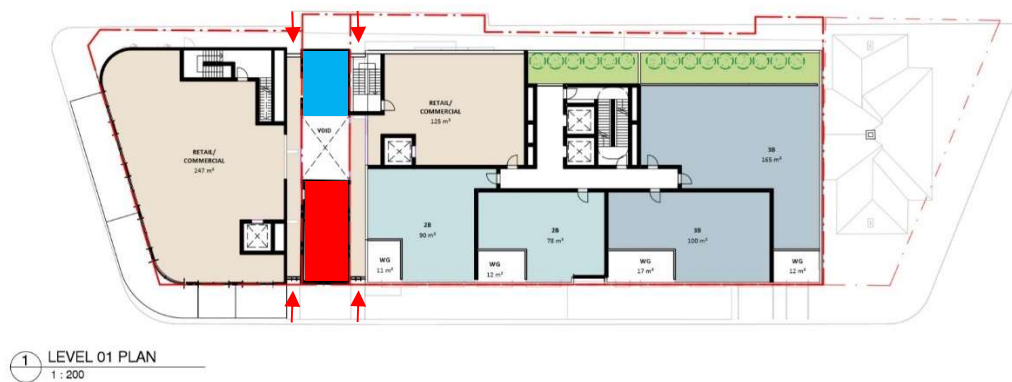
Figure 72 - Plan showing the heritage item (shaded red) integrated into the level 1 planning, including the proposed structure (shaded blue) at the rear of the site and courtyard (void) between. Note also the indents (see red arrows) marking the location of the heritage item on both the Pacific Highway and Church Lane elevations. (Source: PTW Architects)
